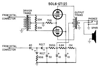
Cure: A scope check was made on the power amplifier chassis, and the trouble was isolated to a intermittent connection in the center tap of the driver transformer. Replacing this transformer cured the trouble.—George P. Oberto
